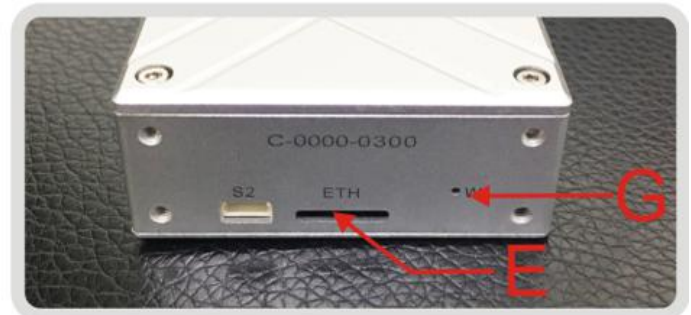
E: 1*100Mbps Ethernet G: WL Signal Indicator
