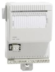
The DO801 is a 16 channel 24 V digital output module for the S800 I/O. The output voltage range is 10 to 30 volt and the maximum continuous output current is 0.5 A. The outputs are protected against short circuits, over voltage and over temperature. The outputs are in one isolated group. Each output channel consists of a short circuit and over temperature protected high side driver, EMC protection components, inductive load suppression, output state indication LED and optical isolation barrier.
